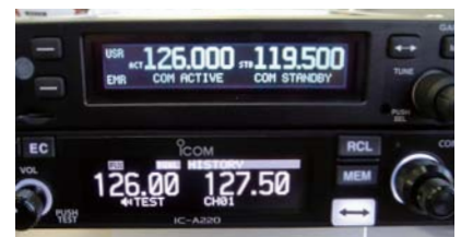
Display comparison with a competing product (IC-A220 is below) Its flip-flop key is large and prominent.
